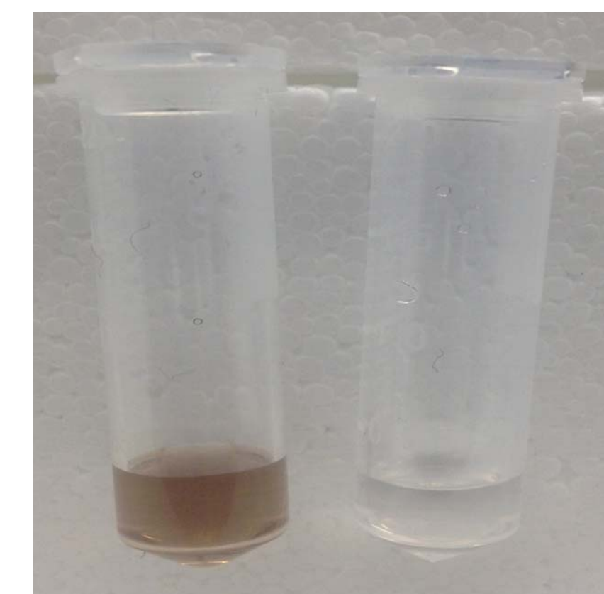
Figure 6: Supernatant from loaded O-GNR coated with 6K (l) and 10K (r) Dextran
